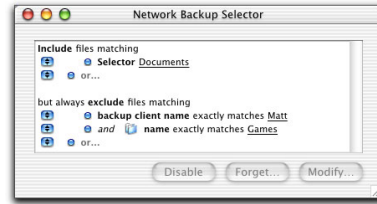
A network backup selector that excludes a specific folder on a specific client computer.
